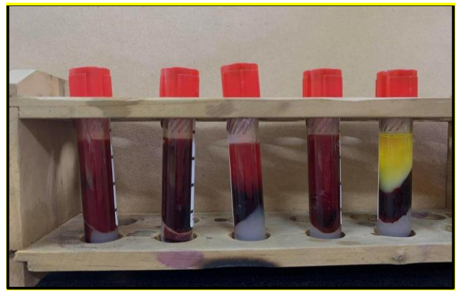
Fig. 3. Serum separation resulting from adding 0.22 g/mL I. batatas starch gel
